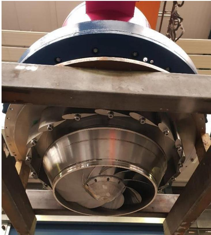
Factory acceptance test of the turbine generator unit
